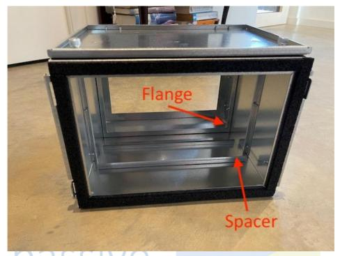
I used some simple T section aluminum strips to provide a 'track' for the HRW side of the filter to keep the filter in place and square against the new rubber seals. The aluminum strips were riveted in place and foil tape used to cover the rivets avoiding any possible air leakage and or noise.
